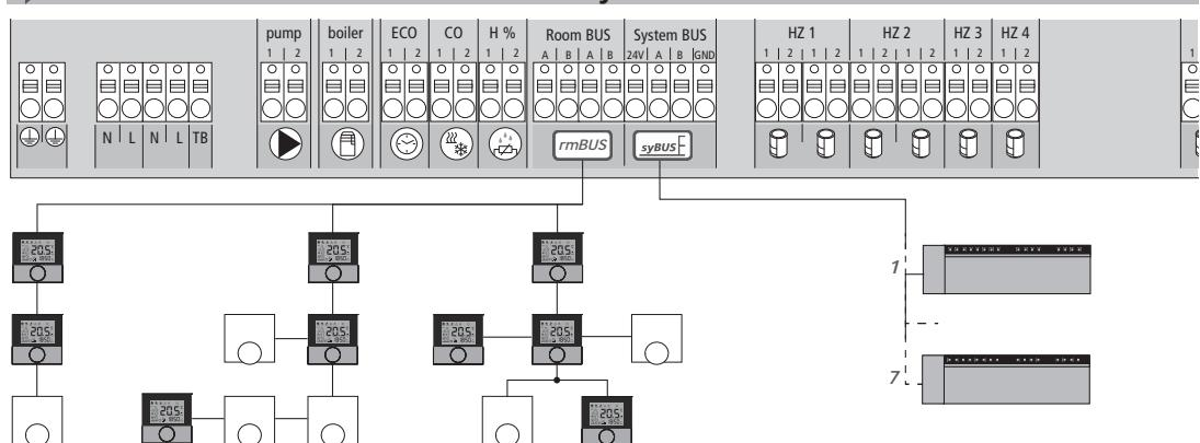
Depending on the type of base station, a maximum of four, eight or twelve room control units can be connected to the Room Bus. The connection of the room control units can be executed in the topologies "line", "tree", or "star". A maximum of seven base stations can be coupled with the System Bus. A solid wire 2x2x08 must be used for wiring. For a line diameter <6 mm, a strain relief must be provided by the customer.
