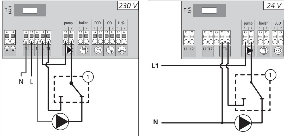
Connection of a customer-supplied safety temperature limiter (1). This device switches off the pump and sets the input to TL if too high flow temperatures for the floor heating are detected. If the TL input is switched, the base station shuts down all actuators automatically.
