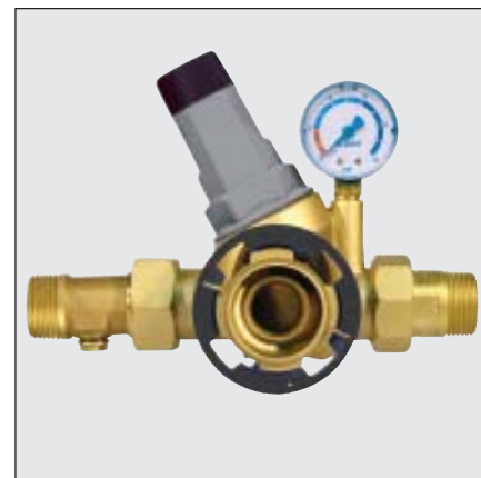
HWS connecting module with pressure reducer and non-return valve
