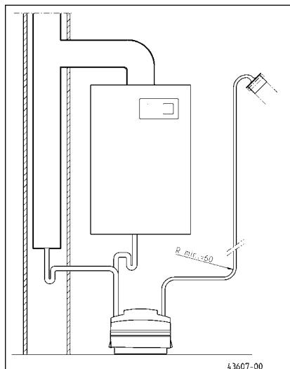
**ATTENTION!** The pressure line, from its highest point, must be able to completely discharge its contents. Pockets of air in the pressure line increase the pumping resistance.
